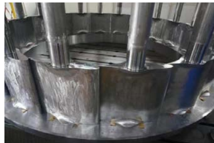
Fig.2 Vane after Manual Welding and Grinding
